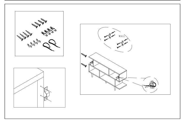
Using a second person to assist you, place the unit in the desired final location against a wall. It is suggested to use a stud finder to find wall studs along the length of the unit and roughly 1 inch below the top of the unit. Where possible, mark a drill hole position on the wall where there is a stud and use a drill or screwdriver (NOT INCLUDED) to attach wall Brackets (A) to the wall using Long Screws (B) in the location of the wall studs.
