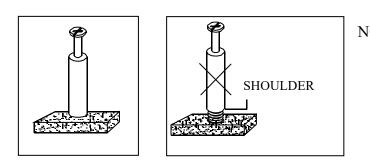
NOTE: • Turn the cam-bolt screws until they are tight, the shoulder should be against the surface of the part.
